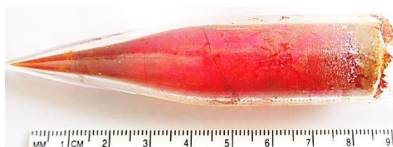
Fig. 1. Photo of as-grown Tl_4HgI_6 single crystal
