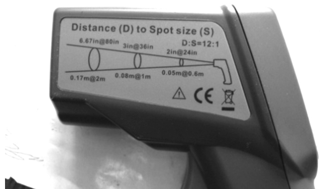
Fig. 16. Laser pyrometer, which was used for the study
